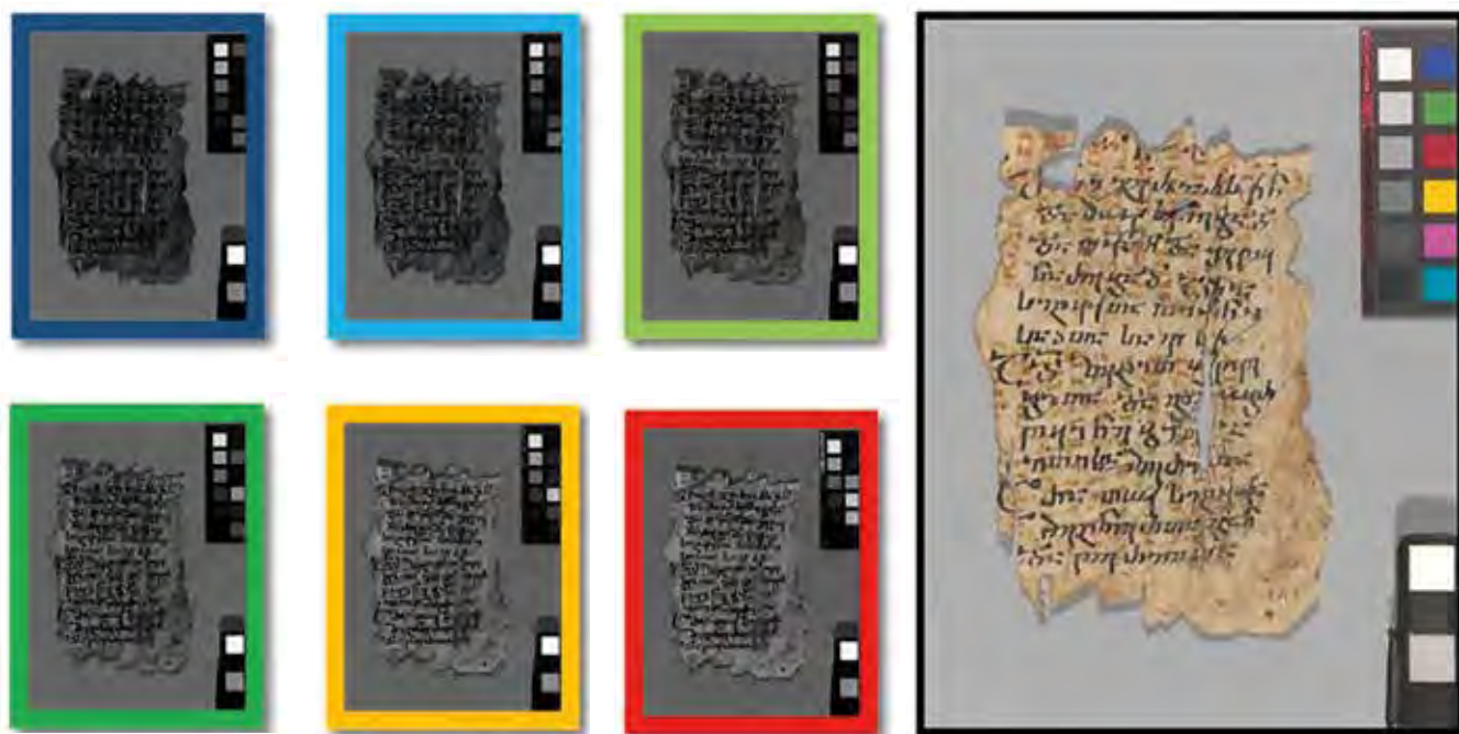
Fig. 2: Color image produced by combination of visible wavelengths. 7 visible wavelengths are used to produce the color image, in this example only 6 pictures are visible for reasons of spacing.
