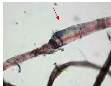
Fig. 19c: A fibre of paper mulberry enveloped by a transparent membrane after being treated with a Herzberg stain. Observed at 400× magnification in manuscript CMRU ARP.TAI 001, the Chiang Mai Rajabhat University Library, Chiang Mai, Thailand.
