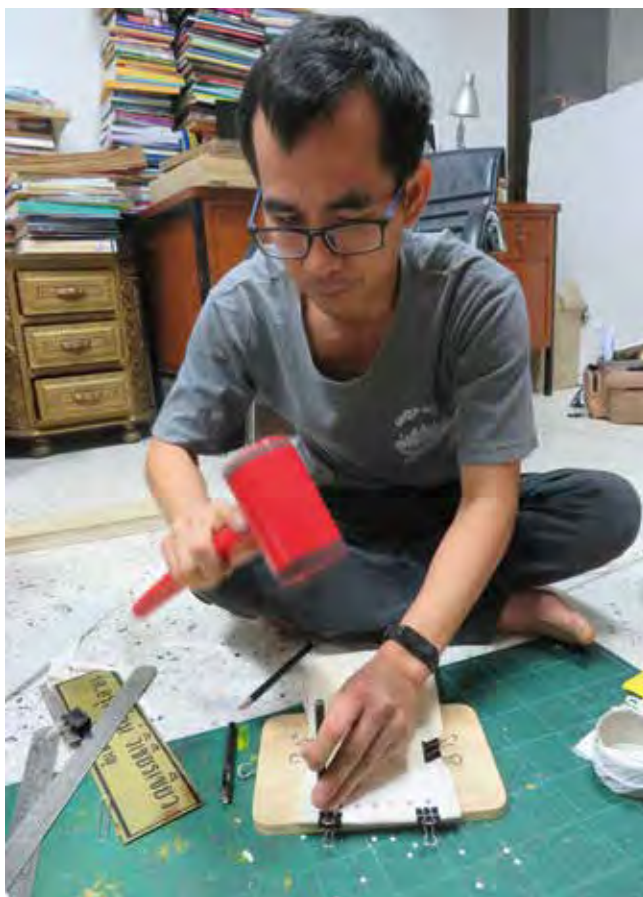
Figs 11a and b: The holes are 'stabbed' by using a sharp metal punch with an eye in it through which a cotton cord is then threaded. The technique is being demonstrated here by Direk Injan from the Chiang Mai Rajabhat University Library in the city of Chiang Mai, Thailand.
