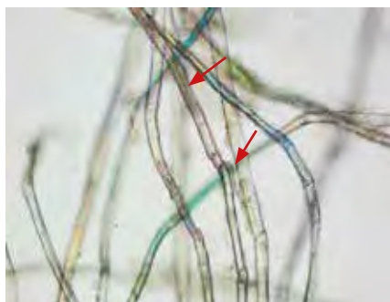
Fig. 19a: The arrows show some thick-walled fibres of paper mulberry enveloped by a transparent membrane. Observed at 200× magnification in the micro-sample from manuscript CMRU ARP.TAI 001 from the Chiang Mai Rajabhat University Library, Chiang Mai, Thailand.
