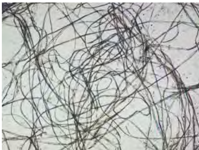
Fig. 18: Well-preserved paper-mulberry fibres observed under the microscope at 40× magnification in manuscript DS 0062 00294 from the Buddhist Archives of Luang Prabang, Laos.
