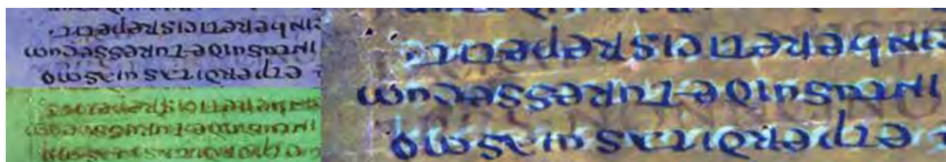
Fig. 14: The ruby image (right) is obtained by dividing a color transmission image (top) by a color fluorescence image (bottom).
