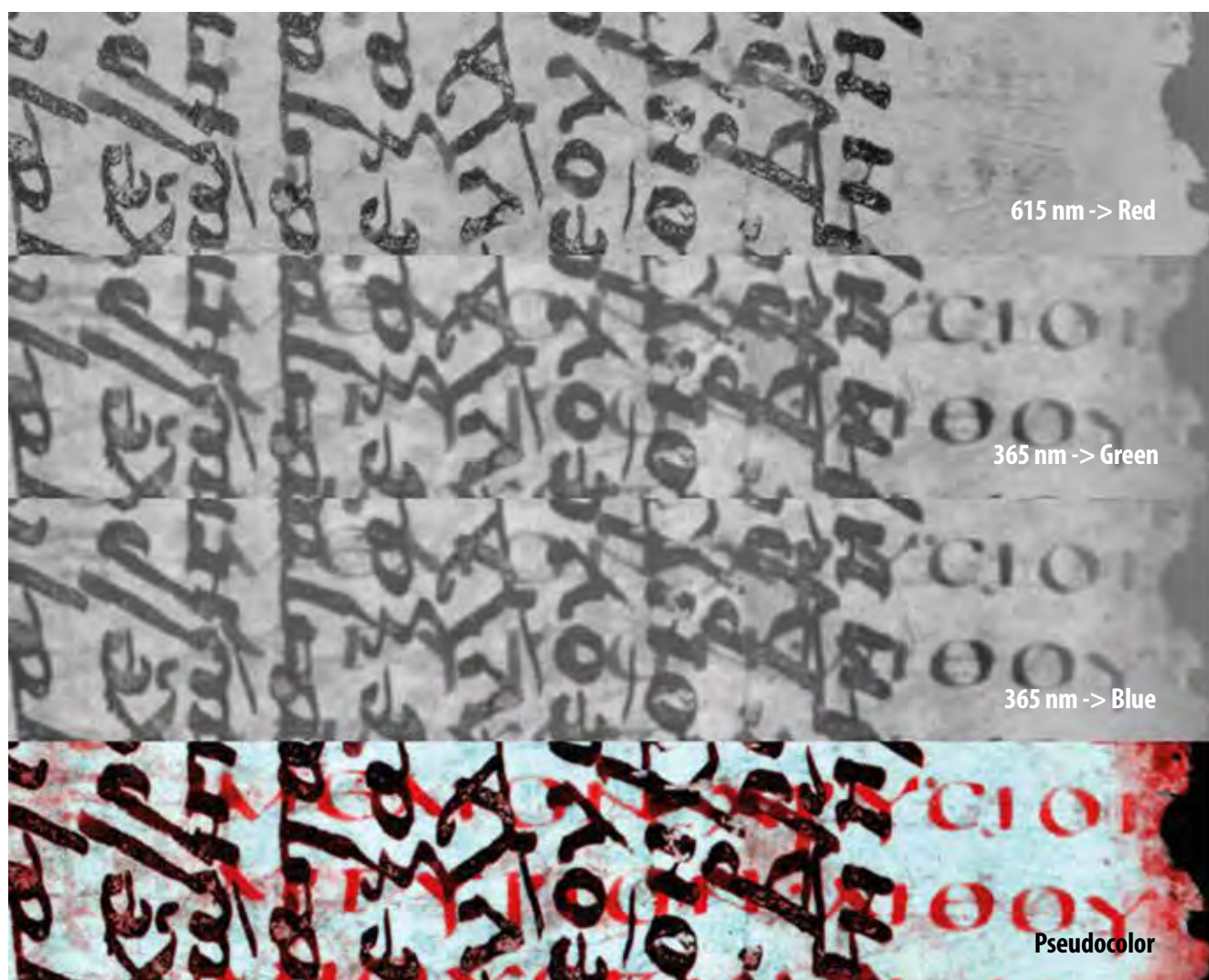
Fig. 4: Greek NF MG 99, fol. 3 v –4 r . A pseudocolor image is created from a visible image, in which the erased text cannot be seen, and a fluorescence image in which both texts are visible.
