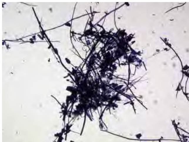
Fig. 22: The bamboo and grass-type pulp observed at 40× magnification in manuscript CMRU Ms. 3 from the Chiang Mai Rajabhat University Library in Thailand.
